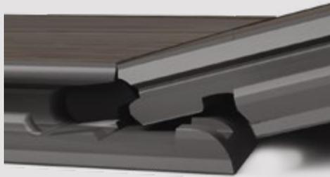
The advanced Välinge 5G installation system makes Rigid fast and simple to fit. Even if you're working in tricky or restricted spaces, you can easily achieve a perfect finish. Push down end joints need less positioning space, so there's no need to remove doors whilst fitting. 5G provides stronger and more stable end joints too.
